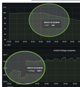
Figure 2 : Voltage increases during discharge controlled by the Studer Innotec NEXT3 inverter
