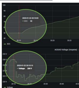
Figure 4 : Voltage reduction during charging controlled by the Studer Innotec NEXT3 inverter
